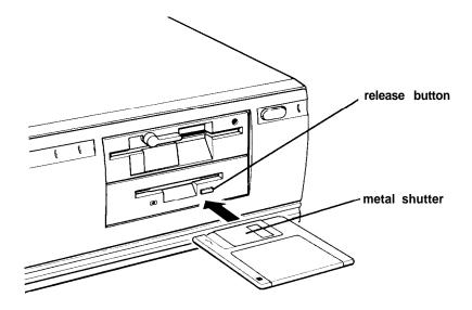
When you want to remove the diskette, make sure the drive light is off; then press the release button. When the diskette pops out, remove it and store it properly.
